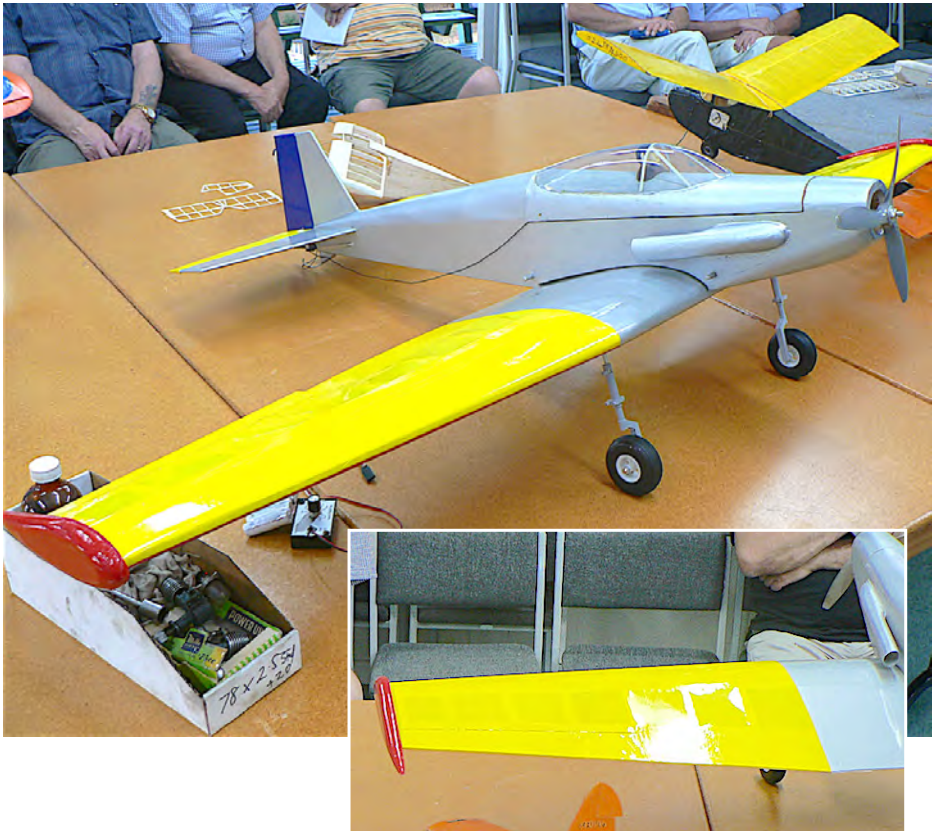
Upper and inset: Charles Warren's latest version of his Turbo showing functional ducts for motor cooling and knock-off wing tips.
